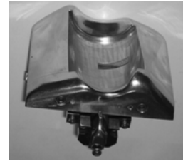
Fig. 1. The component and the whole assembly of the template for rotor winding
